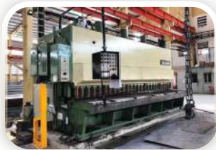
Steel Plate Cutting (16/22mm- 4/6m)
