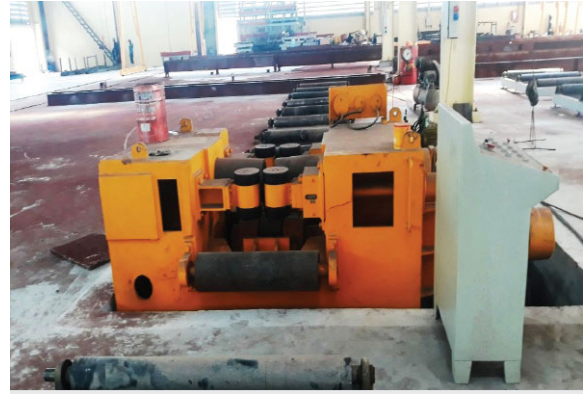
Beam bending machine
